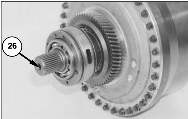
7. Remove shaft (7) from the torque converter.
