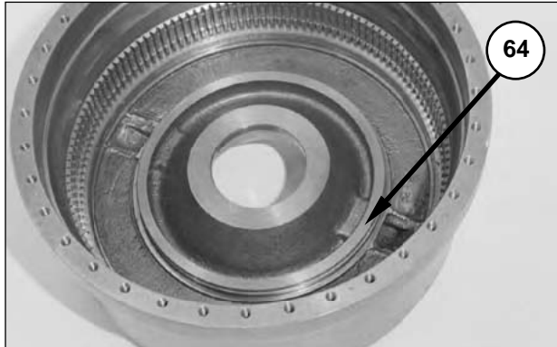
1. Install ring (45) in housing (35).
