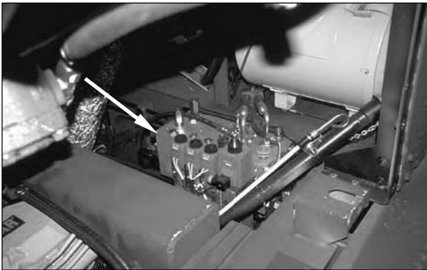
Multifunction Control Valve, Left Side of Machine.
