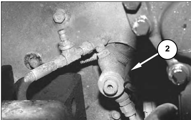
Front of Machine, Under Cab, Attached to Brake Pedal. (2) Service brake switch.
