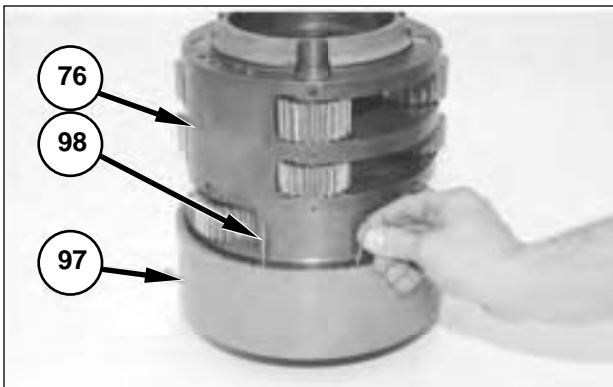
50. Place blocks under planet carrier (76). The blocks will allow ring gear (97) to be removed from planet carrier (76). Use two pin assemblies (98) with a diameter of 3.175 mm (0.125 in) to compress the lock ring. The gear will fall from the carrier assembly.
