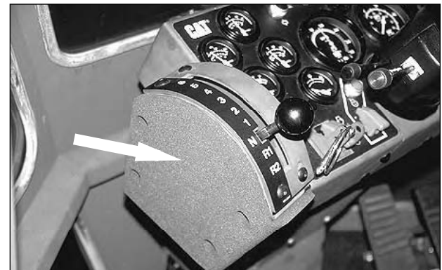
Left Side of Instrument Panel, Switch Located Behind Cover (arrow). (4) Shift lever switch. (5) DEUCE positions.
