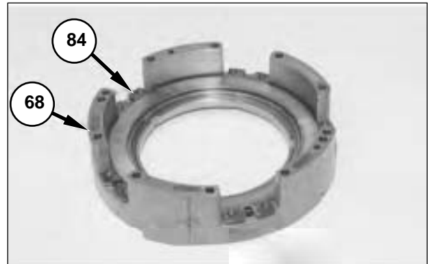
33. Install piston (84) into clutch housing (68).
