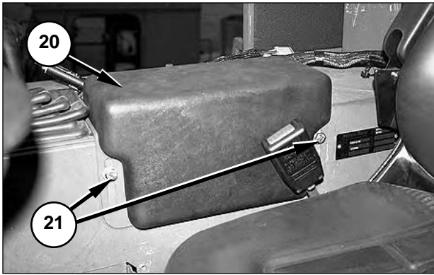
14. Remove two bolts (21) with the washers, and arm rest (20).
