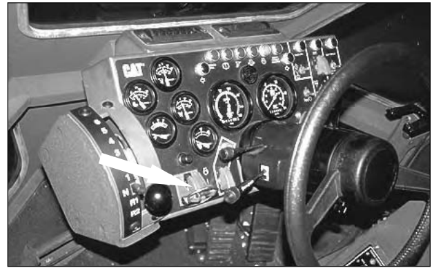
Left Side of Instrument Panel, Switch Located Under Cover (arrow). (12) Engine start switch.
