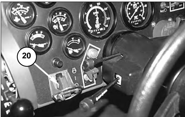
Instrument Panel. (20) Start switch.
