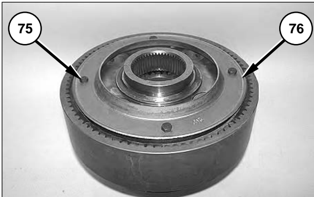
117. Install slinger (76) with four bolts (75).
