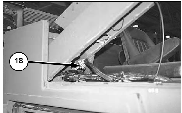
11. Disconnect connector C113 (18).
