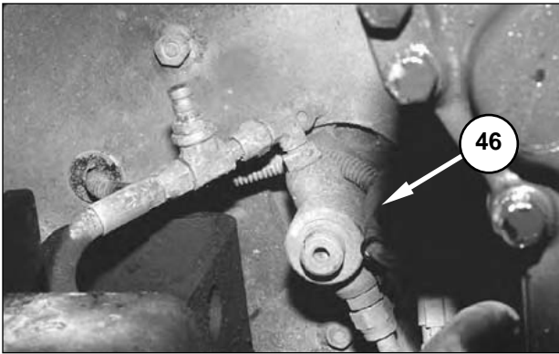
Front of Machine, Under Cab, Attached to Brake Pedal. (46) Service brake switch.
