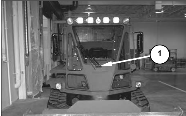
Front of Machine. (1) Wiper motor.
