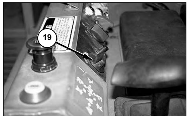
12. Loosen the set screw and remove switch knob (19).
