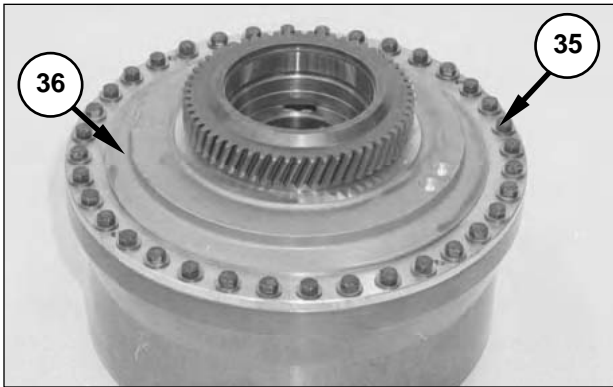
15. Remove 36 bolts (16) and washers, which hold impeller (17) to the housing.
