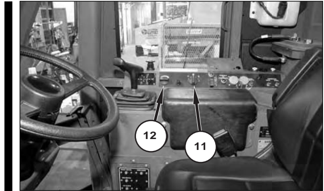
Console to Right of Operator's Seat. (11) Blower switch. (12) Thermostat control knob.
